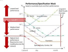
The performance of a TF service is, however, not only determined by the available clocks and oscillators, but also by the TF transfer technique employed. Therefore the network must be comprised of bi-directional TF fibre
