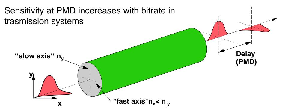
Mod in the SM fiber has two orthogonal polarisations
