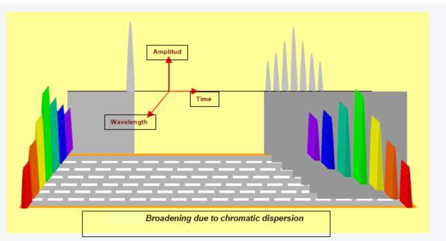
In a positive dispersion fibre, short (blue) wavelengths arrive before long (red) wavelengths. Because laser light sources are not monochromatic, pulse spreading occurs.
